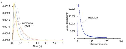
Simulated (left) and experimentally measured (right) particle concentration in room adjacent to emitter
