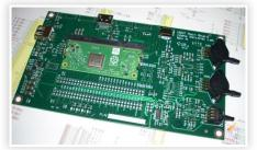
INL IPV ventilator sensor and measurement electronics for Percussionaire Inc.
