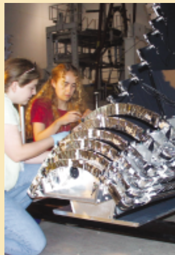
Former Yale graduate student Dan Bardayan, working on a recoil spectrometer and silicon detector array at Oak Ridge.
