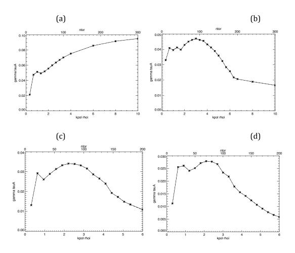
Figure 7. Linear growth rates for the high current Ip=1.13 MA NSTX discharge #128797: (a) using the resistive ballooning mode model, (b) using the diamagnetic stabilization model for the vorticity equation. (c) Adding ad hoc damping near the outer boundaries tames the numerical instabilities that arise at low n, although the peak growth rate is reduced by 30%. (d) Adding ad hoc damping near the inner boundary reduces the peak growth rate by an additional 10%.
