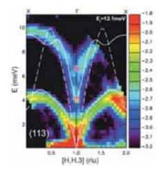
Neutron Scattering Data from the Cold Neutron Chopper Spectrometer at the Spallation Neutron Source. By analyzing the intensities of neutrons scattered from a single crystal of lead telluride, researchers discover an anomalous interaction between phonons moving in different directions, disrupting the flow of heat within the crystal. [Image reprinted by permission from Macmillan Publishers Ltd: From Delaire et al. 2011.]
