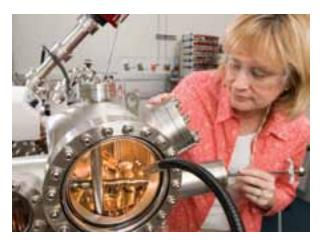
Advanced Instrumentation for New Materials. Kathleen Gregar checks an instrument used to grow pure complex oxide films at the Center for Nanoscale Materials, which supports basic research and instrument development for creating innovative materials with unique functionality. [Courtesy of Argonne National Laboratory.]
