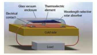
Key Components of a New Solar Thermoelectric Generator for Capturing the Sun's Energy. Encased in a glass vacuum tube to minimize heat loss, the solar absorber soaks up sunlight, which is converted into heat. An electrical current is produced as electrons flow from the hot solar absorber panel to the lower cold side of the device. [Image reprinted by permission from Macmillan Publishers Ltd: From Kraemer et al. 2011.]
