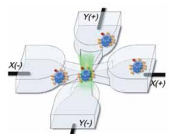
**Investigating the Dynamics of a Single Biomolecule.** Electrokinetic forces compensate for diffusion to trap single molecules of a photosynthetic antenna protein in solution for more than 1 second. [Courtesy of Stanford University.]
