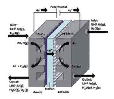
Schematic Cross-Section of the Proton Exchange Membrane Electrolyzer. This new approach uses water vapor instead of liquid water as a feedstock for generating hydrogen
