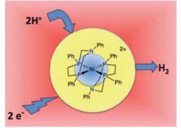
New Synthetic Catalyst for Converting Electrical Energy into Chemical Energy Stored in H<sub>2</sub> Molecules. The new complex uses nickel (Ni) instead of more expensive metals like platinum to set record-breaking conversion speeds that outperform natural enzymes. [Courtesy of Pacific Northwest National Laboratory.]
