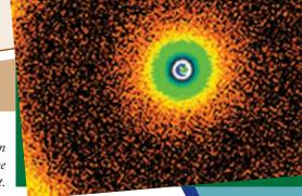
Two-dimensional scattering pattern of a polymer from data taken at the Bio-SANS instrument.
