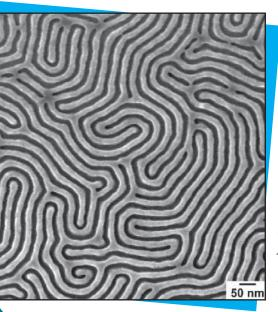
Scanning electron microscope image of a lamellar-phase block copolymer thin film. This self-assembled striped pattern has feature sizes of 18 nanometers with 36 nanometer period spacing.
