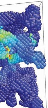
Computer generated model of a copper nanofoam deformed under volume conserving planar strain.
