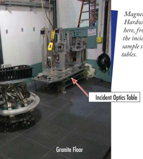
Magnetism Reflectometer. Hardware items depicted here, from right to left, are the incident optics, hexapod sample support, and detector tables.
