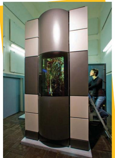
The world-leading monochromated, aberration-corrected TEAM 0.5 microscope is capable of half-Angstrom imaging in both, broad-beam and scanning-probe modes of operation.
