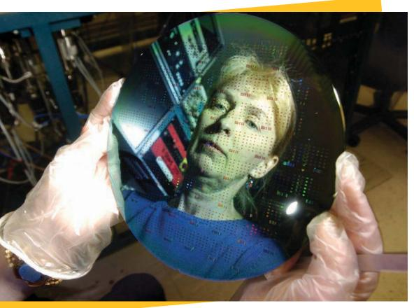
IBM researcher Simone Raoux with a wafer that contains millions of new computer memory switches. Raoux performs research partly with time-resolved x-ray diffraction at the NSLS to develop a material that could lead to a new kind of computer memory chip used for storing digital media. Photo courtesy of Noah Berger/The New York Times/Redux.
