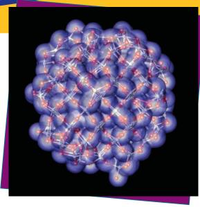
Structure and charge density of a 2-nm titanium dioxide nanoparticle from ab initio calculations. (Courtesy of Paul Kent, Oak Ridge National Laboratory, and James Kubicki, Penn State University.)
