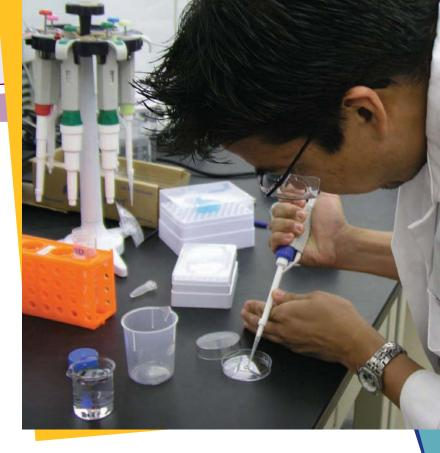
Preparing a slide of quantum dot attached microtubules for an atomic force microscopy experiment.
