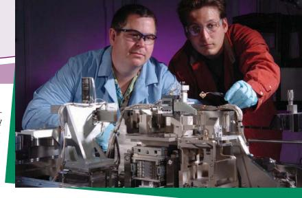
The CNM hard x-ray nanoprobe beamline provides fluorescence, diffraction, and transmission imaging, both static and dynamic, with a spatial resolution of 30 nm or better over a spectral range of 3-30 keV. The Fresnel zone plate being placed in the beam path by facility scientists Martin Holt, next to Robert Winarski, focuses the x-ray beam using a series of nanometer-sized concentric rings etched into the gold sheet.
