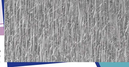
Forest of GaN nanowires grown by MOCVD on a saphire substrate using a Ni catalyst. The nanowires are about 100 nm in diameter.
