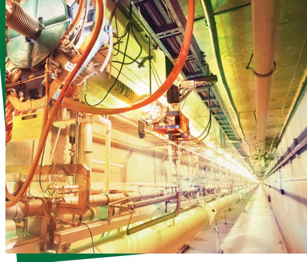
The SLAC linear accelerator will accelerate pulses of electrons to nearly the speed of light, and use them to create extremely intense, coherent pulses of x-rays through the free-electron laser process.
