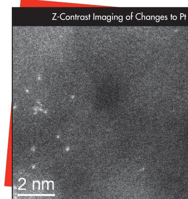
In the first image, single Pt atoms in fresh catalyst appear as white dots ~ 1Å in diameter. After reduction treatment to enhance catalytic activity, the second image shows these Pt atoms forming small (<2nm) clusters.
