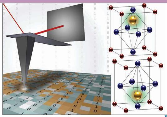
Scanning probe microscopy-based manipulation of local polarization in ferroelectric materials enables studies of bias-induced phase transitions on a single-defect level, and can also serve as the physical basis of ultrahigh-density information storage. Related techniques may be used to probe electromechanical energy conversion mechanisms and electrochemical reactions on the nanoscale. (Courtesy of Stephen Jesse and Sergei V. Kalinin, CNMS, Oak Ridge National Laboratory.)
