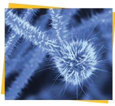
Cu-TCNQ nanowires on ZnO nanowires. Here TCNQ is the common abbreviation for 7,7,8,8-tetracyanoquinodimethane, an organometallic semiconductor charge transfer material. (Courtesy of Kai Xiao, CNMS, Oak Ridge National Laboratory.)
