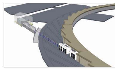
Schematic view of the hard x-ray nanoprobe beamline, with a remote satellite building at ~100 m from the source.
