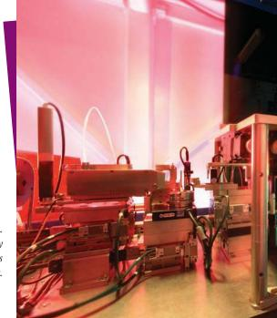
Transmission X-ray Microscope installed at SSRL BL6-2. This instrument is the heart of an NIH funded, hard x-ray bio-imaging facility capable of resolutions of 40 nm as well as tomography in both phase and absorption contrast.
