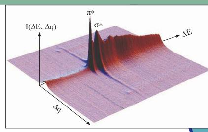
High-resolution momentum resolved spectroscopy developed within the EMC allows researchers to investigate the orientation dependence of the electronic properties of materials.
