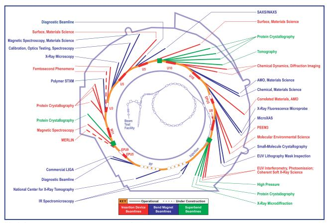
The ALS can operate 35 beamlines simultaneously for its users. In addition, six beamlines are in the commissioning or advanced construction stage—three based on undulator sources, two on normal bend magnets, and one on a superbend magnet.
