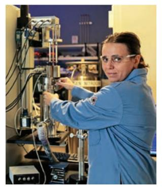
**Developing Complex Materials with Enhanced Properties.** Vera Bocharova, of Oak Ridge National Laboratory (ORNL), performs broadband dielectric spectroscopy, a technique capable of capturing a variety of material synthesis mechanisms and phenomena by probing temperature-dependent dynamics on time scales from 10<sup>-8</sup> to 100 seconds. [Courtesy ORNL]
