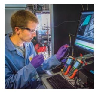
**Examining a Solar Fuels Generator Prototype.** JCAP scientist Karl Walczak tests and evaluates the performance of a hydrogen solar fuels generator under simulated sunlight. [Courtesy Lawrence Berkeley National Laboratory]
