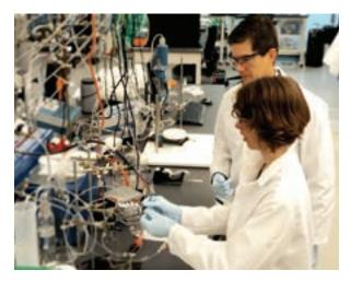
**Converting Carbon Dioxide to Fuels and Chemicals.** Stephanie Nitopi, a Stanford University graduate student, and Professor Thomas Jaramillo set up a carbon dioxide reduction experiment in the Jaramillo group's custom electrochemical cell. [Courtesy SLAC National Accelerator Laboratory]
