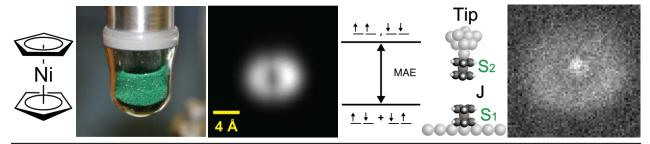
An example of a magnetic molecule nickelocene (NiCp2), showing the schematic structure, greenish bulk solid and STM topographic image, as a qubit of the superposition of the m=0 and m=±1 states separated by the magnetic anisotropy energy (MAE); two qubits (one on the STM tip and another on the surface) and the spatial distribution of the exchange energy J(x,y).
