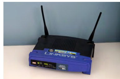
Figure 7: The WRT54g, an open, customizable wireless device.
