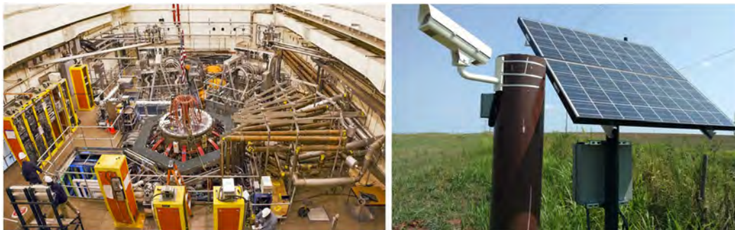
Figure 8: From the experimental hall to the field site, advanced wireless, including 5G, will revolutionize the configuration of sensor networks. The left panel shows the next National Spherical Torus Experiment Upgrade experiment with high-speed data collection needs. The figure on the right, courtesy of Rusen Oktem (LBNL), shows one of a pair of stereo cameras [66] deployed to the ARM [8] Southern Great Plains site in Oklahoma.
