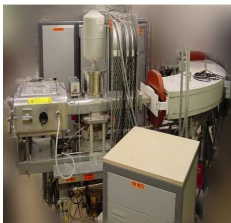
Figure 12: INL stable mass separator
