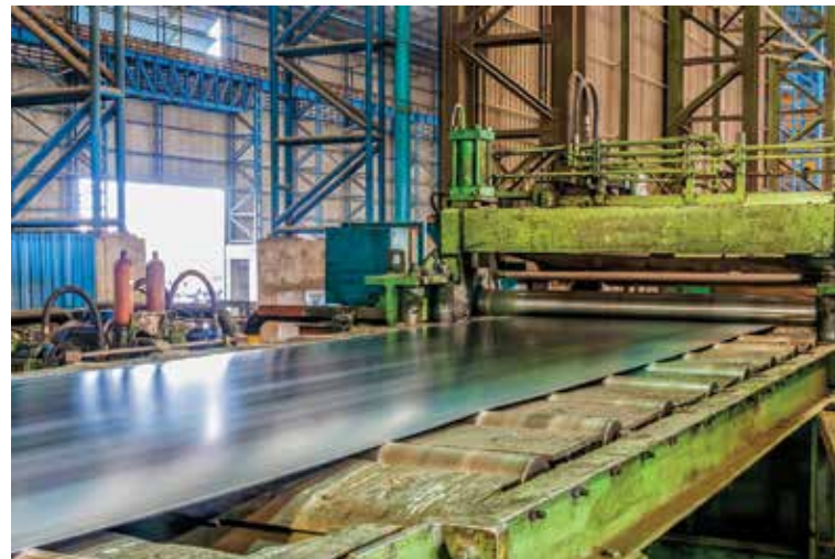
Top: Hot metal cooling after casting. (Tdhster / Shutterstock.com) Bottom: Rolling mill processing steel plate. How metals are processed affects their microstructure and hence their properties. (Sayam Trirattanaipoon / Shutterstock.com)
