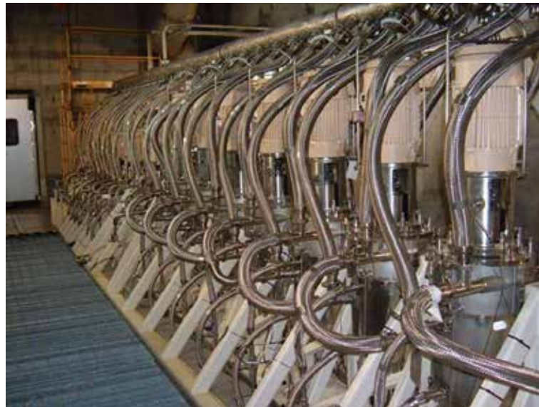
Solvent extraction equipment used at the Savannah River Site to separate radioactive cesium from legacy nuclear waste. (U.S. DOE Savannah River Site)
