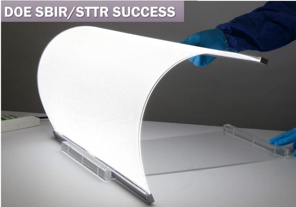
Lucent Optics' advanced light coupling technology allows for injecting light from LEDs into thin light-guiding sheets, producing low-cost, large-area, flexible lighting panels.
