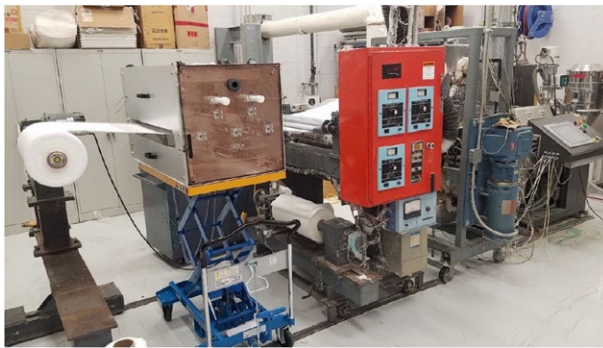
Fig. 5.18. Corona charging system integrated at Cummins Inc. [Courtesy Oak Ridge National Laboratory]
