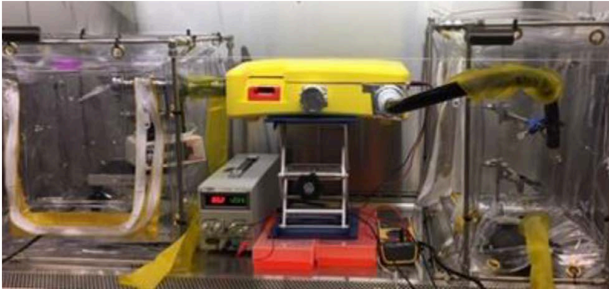
Fig. 5.30. Experimental setup for testing microbial deactivation as part of efforts to develop filtration systems for breathing hoods. [Courtesy Savannah River National Laboratory]
