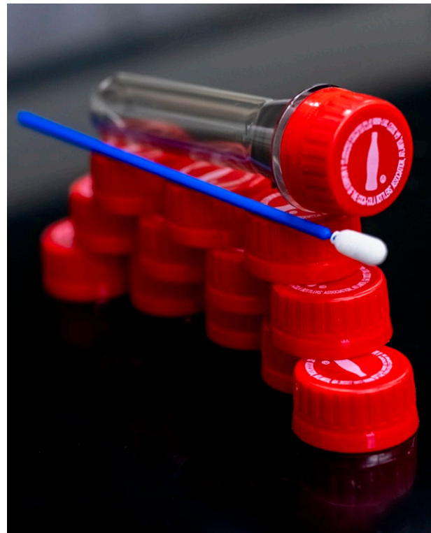
Fig. 5.7. A Coke bottle preform with Coke lids used as substitutes for sample collection tubes. [Courtesy Oak Ridge National Laboratory]
