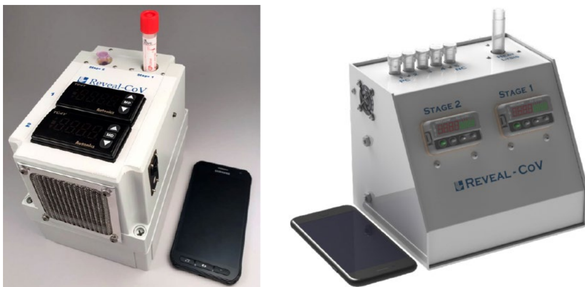
Fig. 2.31. Reveal-CoV instrument development. First unit build of prototype single assay instrument consisting of two single-tube heaters for sample inactivation (Stage 1) and detection assay amplification (Stage 2) [left]. CAD model of five assay instrument concept consisting of a sample inactivation heater (Stage 1) and a 5-tube detection assay heater (Stage 2) [right]. [Courtesy Lawrence Livermore National Laboratory]
