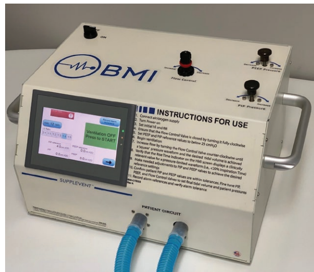
Fig. 5.59. The final ventilator product showing the user interface and knobs to control power, flow, PIP, and PEEP. The blue tubes are the air pathways to and from the patient. [Courtesy BioMedInnovations, LLC]
