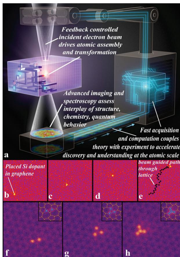
**Figure 5.** (a) Enhanced STEM enables building and editing of atomic assemblies and assessment of their quantum properties. (b–e) Directed doping and guided motion of dopant through graphene lattice. (f–g) Beam-directed atom-by-atom fabrication of silicon dimer, trimer, and tetramer. | Reprinted by permission from Nature Publishing Group. [Nature](#), [Fire up the atom forge](#), S. Kalinin, A. Borisevich, and S. Jesse, copyright 2016
