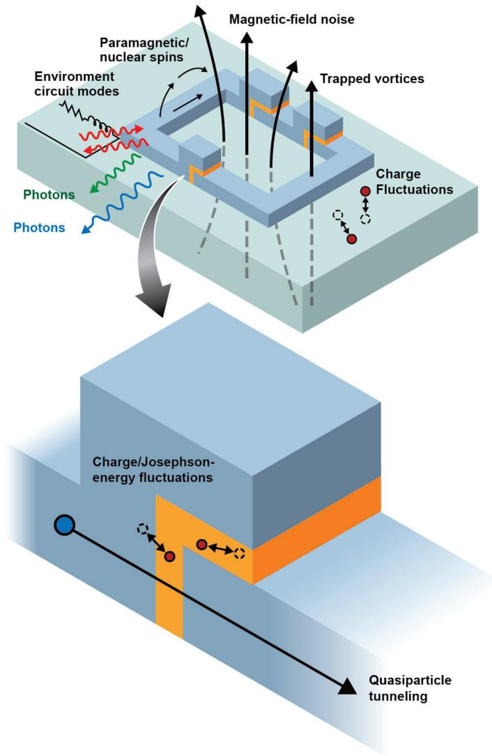
**Figure 11.** Illustration of various decoherence mechanisms that can affect superconducting qubits. The mechanisms include those related to materials and fabrication, as well as design and packaging considerations (environmental circuit modes and photons). | Image from W. D. Oliver and P. B. Welander, [Materials in superconducting quantum bits](#), *MRS Bulletin* 38(10), 816–825, 2013, copyright 2013 by Cambridge Core. Reproduced with permission
