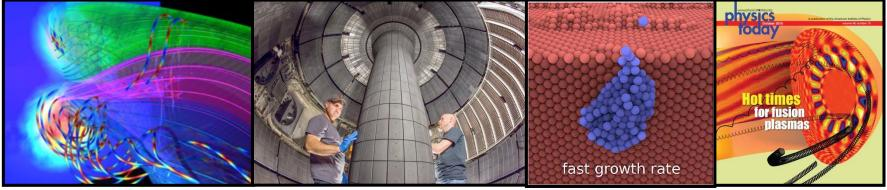
Magnetic reconnection driven by 3-D flux-rope interaction in the Large Plasma Device New central solenoid magnet inside NSTX-Upgrade Growth of helium bubbles that degrade tungsten performance
