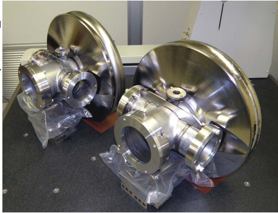
Superconducting electron gun, developed at BNL by DOE in cooperation with DOD and industry.
