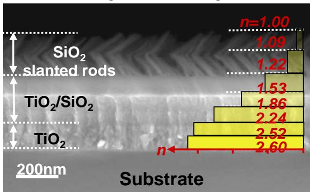
SEM Image of a 7-layer graded anti-reflection coating structure
