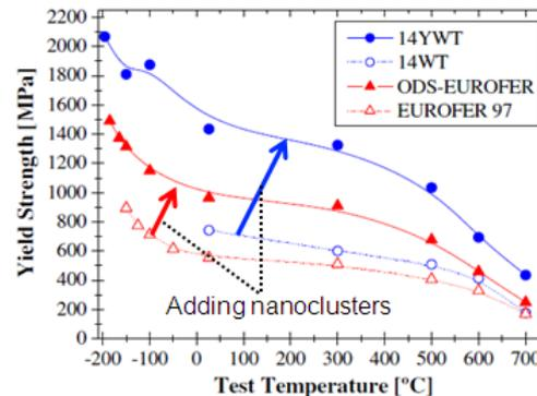
Stable nanoclusters (~2-4 nm in size) are found in ferritic alloys prepared by mechanical alloying and serve to increase strength even after long times at high temperatures
