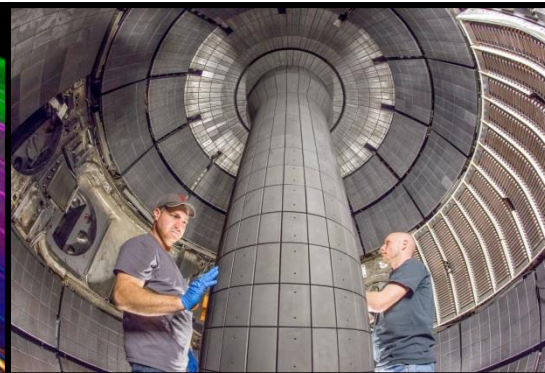
New central solenoid magnet inside NSTX-Upgrade
