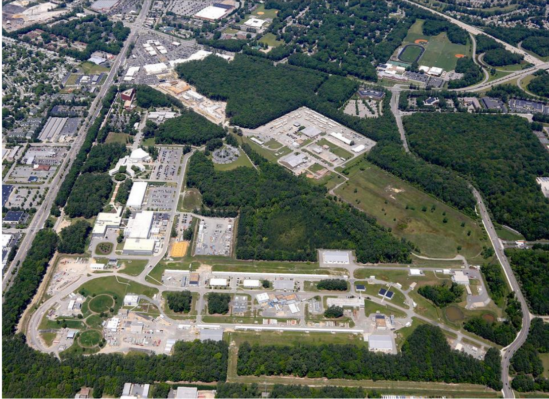
View from flyover of Jefferson Lab, facing towards the north. The racetrack outline of the Lab's accelerator facility is located in the southern portion, while the experimental halls are located at the eastern and western ends of the accelerator loop.
