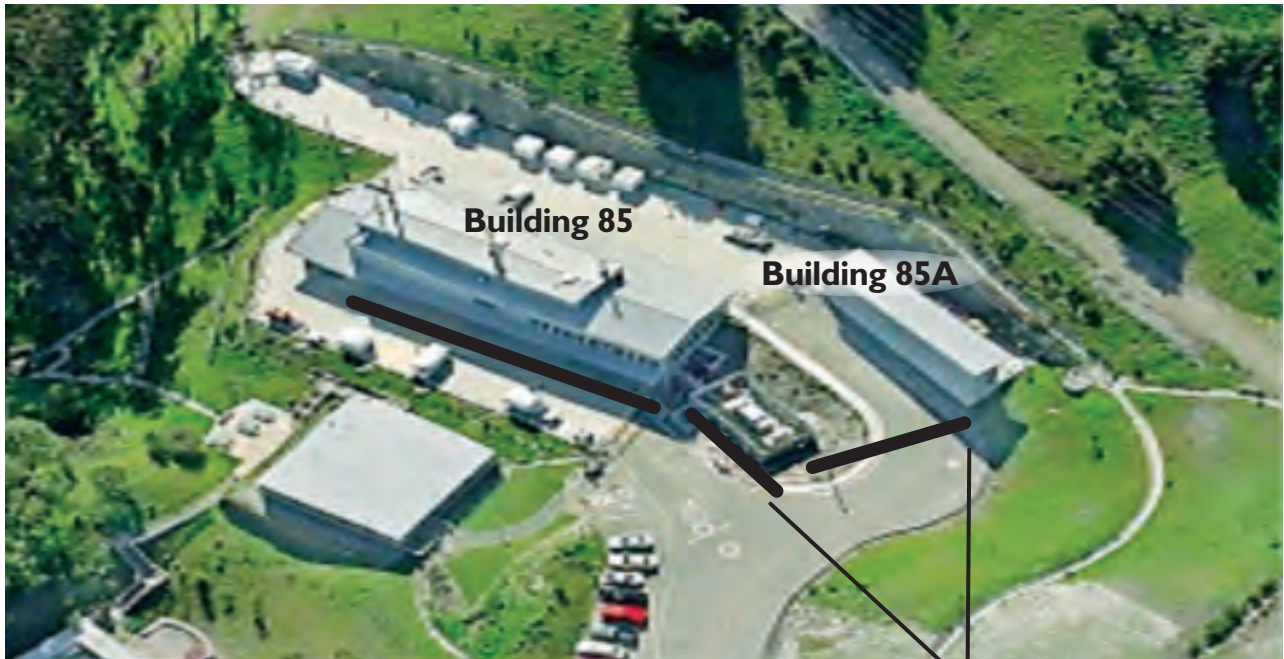
Proposed locations for underground retaining structures, such as pier foundations and tie backs
