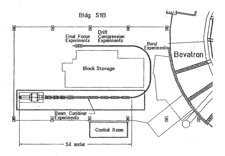
Figure 4. Overall Induction Linac System Experiments Configuration
