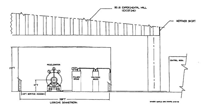
Figure 3. Cross-section View of the Proposed Building and Accelerator Area in Relation to Existing Building 51B
