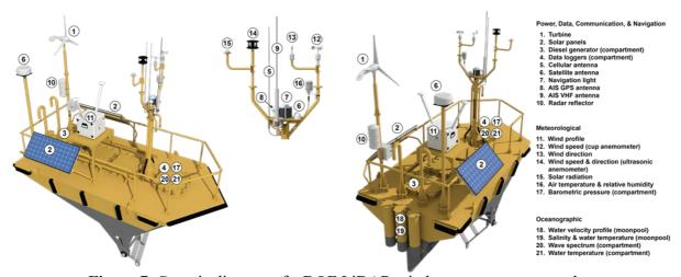
Figure 7. Generic diagram of a DOE LiDAR wind resource assessment buoy.
