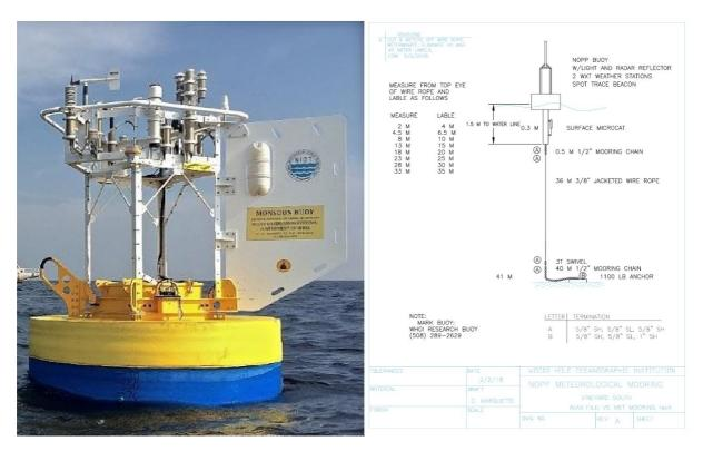
**Figure 9.** (left) Generic diagram of the WHOI sentinel LiDAR buoy, (right) generic mooring design for the WHOI sentinel buoy array.
