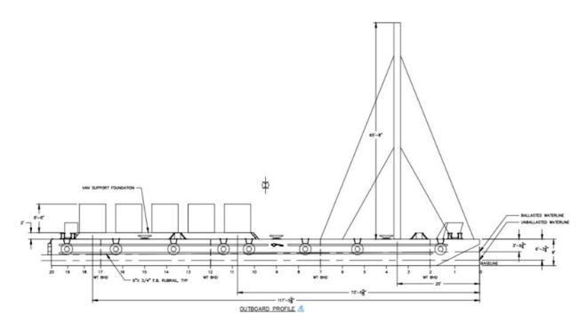
**Figure 6.** Schematic of the Barge with Met mast and science vans (i.e., shipping containers).
