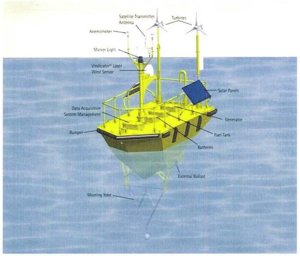
Figure 5. Generic diagram of a WindSentinel<sup>TM</sup> LIDAR wind resource assessment buoy
