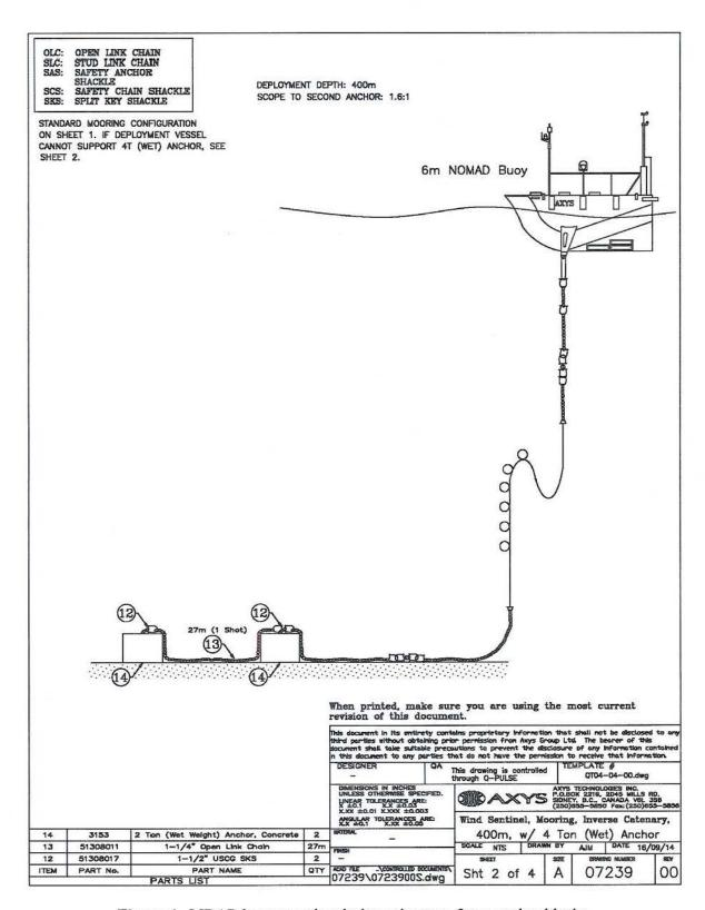
Figure 4. LIDAR buoy mooring design using two, 2-ton anchor blocks.
