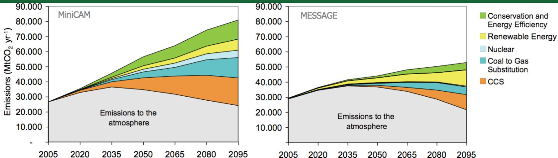
Two scenarios for reducing carbon dioxide emissions to keep atmospheric concentrations at 450-750 ppmv. Left: high-emission scenario, where nuclear plays an important role. Right: low-emission scenario. In both cases, carbon capture and storage (CCS) – the orange wedge – plays a critical role. (IPCC report, 2007)
