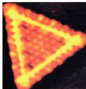
TEM image of a model molbydenum disulfide catalyst showing layers that are only a few atoms across
