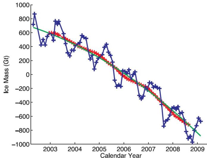
**Figure 1.** Time series of ice mass changes for the Greenland ice sheet estimated from GRACE monthly mass solutions for the period from April 2002 to February 2009. Unfiltered data are blue crosses. Data filtered for the seasonal dependence using a 13-month window are shown as red crosses. The best-fitting quadratic trend is shown (green line). The GRACE data have been corrected for leakage and GIA.
