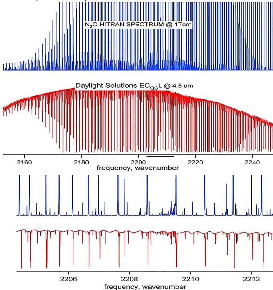
Data plot showing the excellent agreement between an N<sub>2</sub>O mid-IR high-resolution absorption spectrum recorded using Daylight Solutions’ CW-Mode-Hop-Free laser and the NIST ‘HITRAN’ database spectrum.
