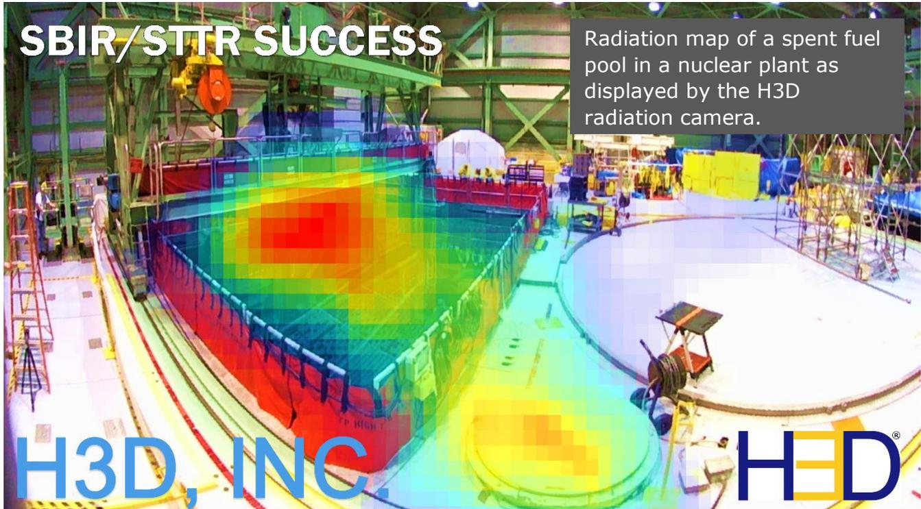
Radiation map of a spent fuel pool in a nuclear plant as displayed by the H3D radiation camera.
