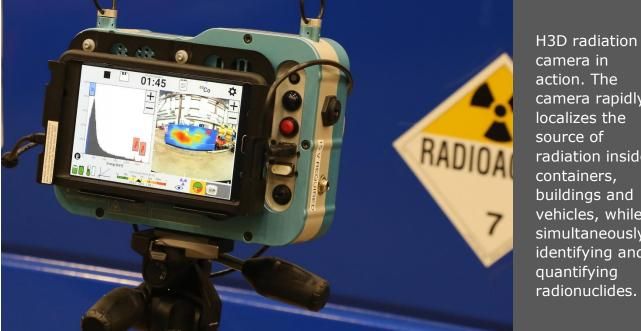
camera in action. The camera rapidly localizes the source of radiation inside containers, buildings and vehicles, while simultaneously identifying and quantifying radionuclides.
