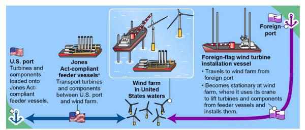
Figure 13: Example of Offshore Wind Installation in U.S. Waters Using a Foreign-Flag Installation Vessel and Jones Act-compliant Feeder Vessels Source: GAO, December 2020<sup>34</sup>
