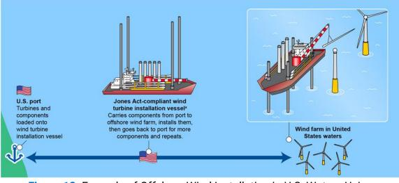
Figure 12: Example of Offshore Wind Installation in U.S. Waters Using a Jones Act-compliant Installation Vessel Source: GAO, December 2020<sup>33</sup>
