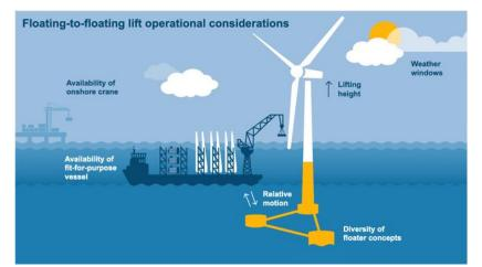
Figure 6: Lifting needs when transferring from one floating entity to another Source: World Forum Offshore Wind<sup>23</sup>
