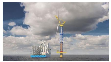
Figure 16: WindSpider Pro Source: WindSpider<sup>46</sup>
