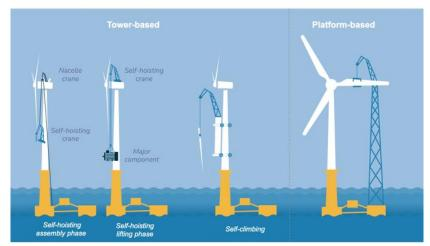
Figure 7: Tower-based and Platform-based Add-on cranes Source: WF0<sup>24</sup>
