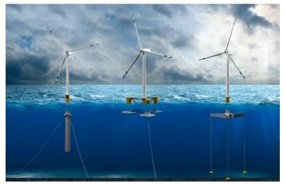
**Figure 4:** Illustration of floating foundation types (NREL 2022) Key, left to right: spar, semi-submersible, TLP **Source:** U.S. Department of the Interior, Bureau of Ocean Energy Management (BOEM), January 2023<sup>11</sup>
