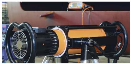
Figure 21: Seifert ERESCO MF4 Portable Industrial X-ray Generator Source: Waygate Technologies<sup>109</sup>
