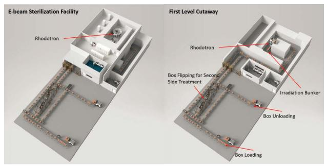
Figure 4: Prototypical E-beam Sterilization Facility<sup>8</sup>
