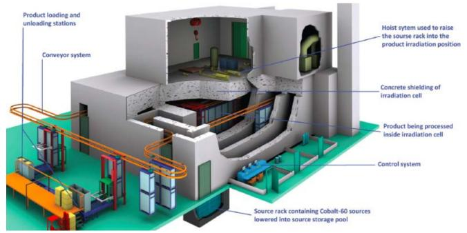
Figure 2: Prototypical Gamma Sterilization Facility Gamma Irradiation Facility<sup>5</sup>
