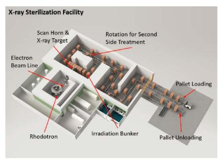
Figure 3: X-ray Sterilization Facility<sup>6</sup>
