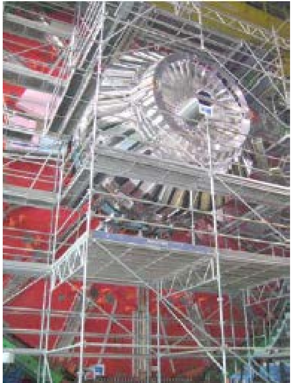
CMS Hadron Calorimeter HE section
