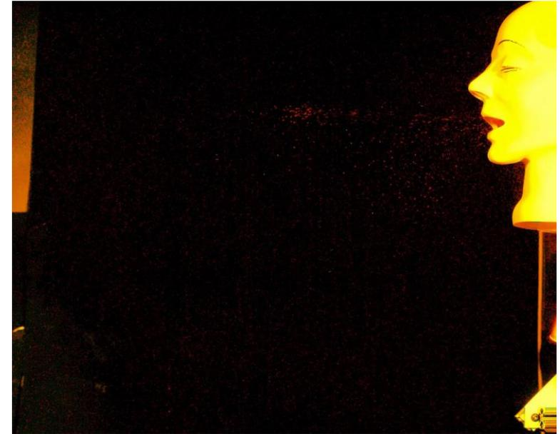
Particles emitted from mouth of a mannequin illustrating different flow paths for different particles
