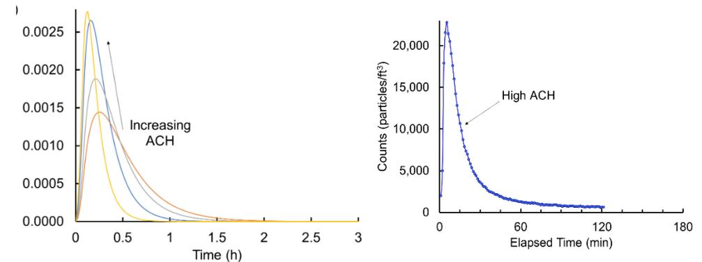
Simulated (left) and experimentally measured (right) particle concentration in room adjacent to emitter
