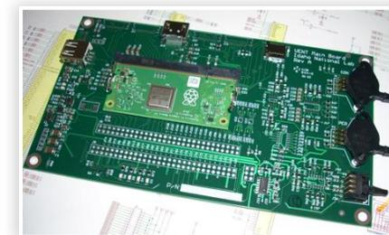
INL IPV ventilator sensor and measurement electronics for Percussionaire Inc.
