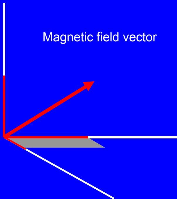
Atomic magnetometers measure length of vector:  $(B_x^2 + B_y^2 + B_z^2)^{1/2}$  by measuring Larmor precession frequency.
