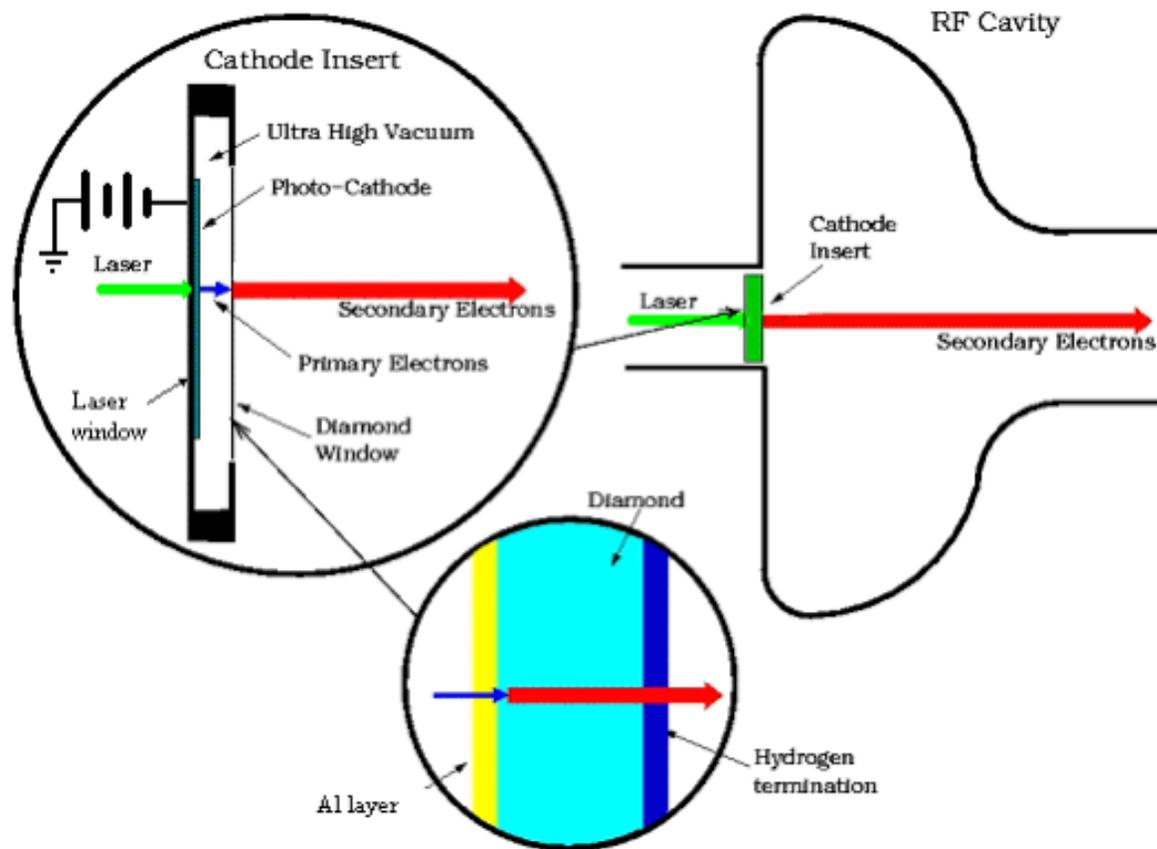
*Schematic diagram of a secondary emission enhanced photoinjector (SEEP)*
