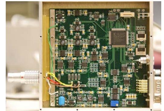
Prototype single-channel feedback loop assembly
