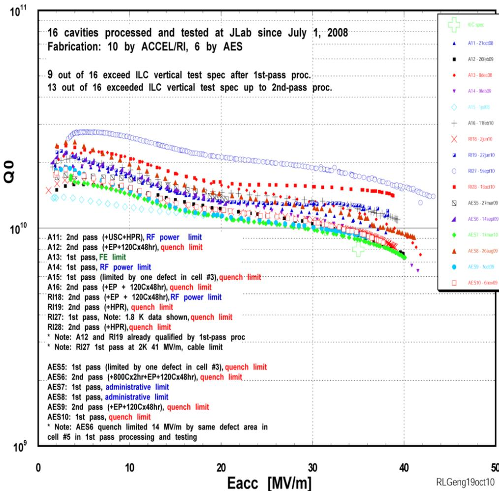
Gradient Yield of 10 ILC Cavities Built by One Vendor Processed and Tested at JLab since July 2008
