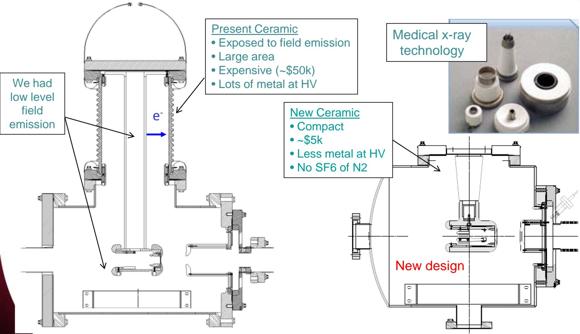
Move away from “conventional” insulator used on most GaAs photoguns today – expensive, months to build, prone to damage from field emission.
