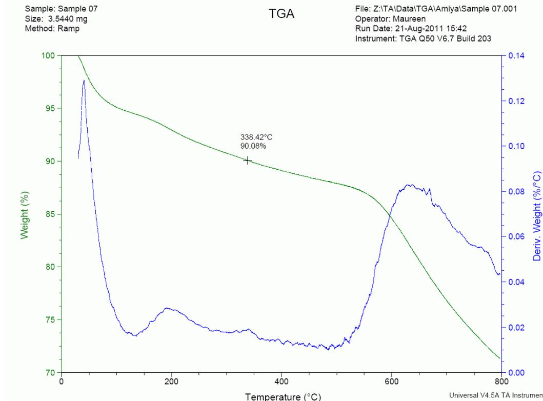
Stripper foil will operate in vacuum. After temperature conditioning, good stability is expected (tested in  $N_2$ , peaks due to water, -OH groups, and possibly oxidation in residual air; TGA Q50).
