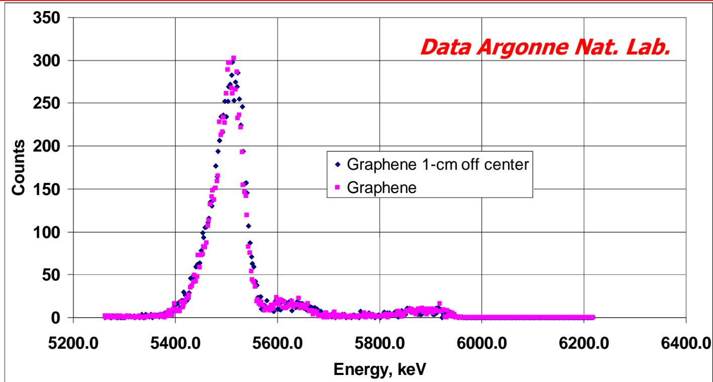
Spectrum of Cf source through graphene foil in the center of the foil and 1-cm off center (foil obtained from U. Wollongong).
