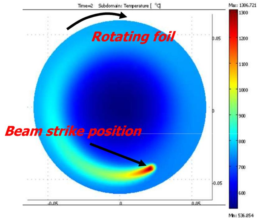
*Calculation of temperature increase of a rotating graphene disk at 1000W dissipated power*
