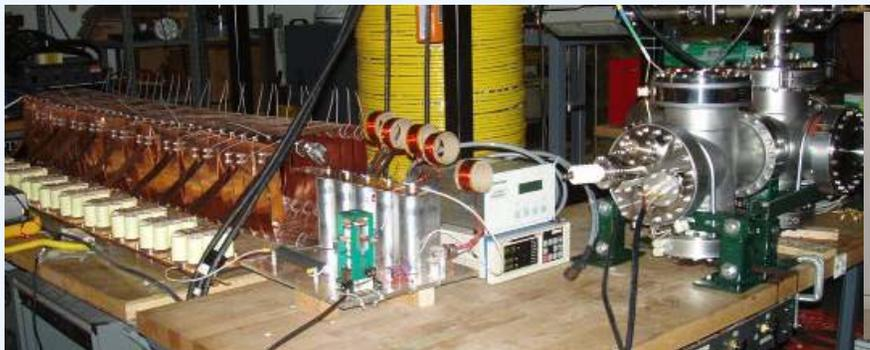
**Cathodic Arc Deposition (CAD)**
