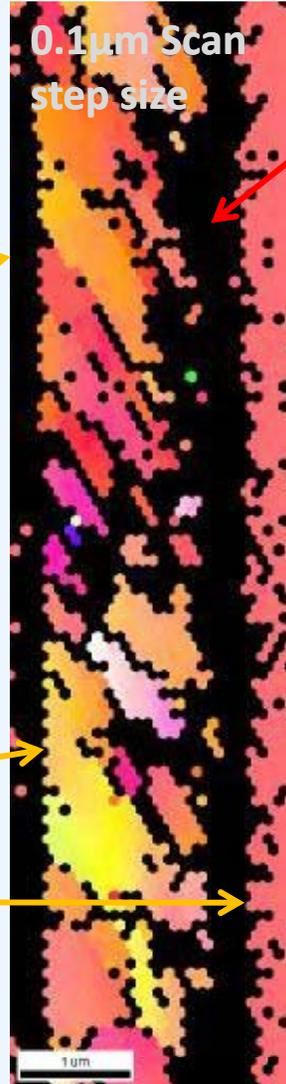
Lower CI values between Nb matrix and MgO substrate indicate that there could be an amorphous or non-structured layer between them
