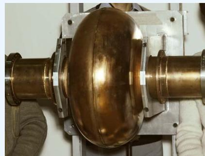
CED<sup>TM</sup> coating of Cu cavities for SRF
