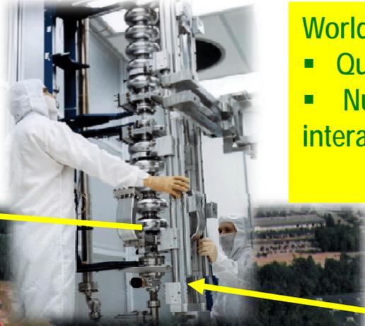
Superconducting radiofrequency (SRF) cavities vertical testing.
