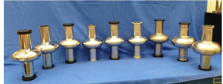
High efficiency, low cost with medium purity (RRR~100) ingot Nb
