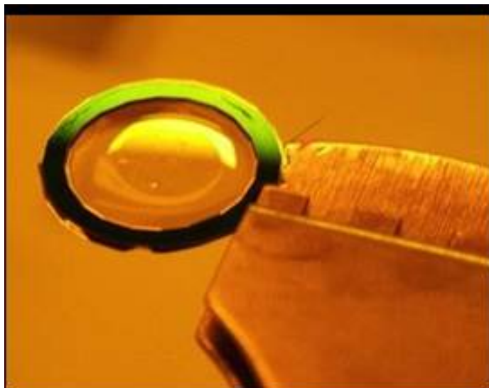
Figure 4: A photograph of a 9mm diameter 200nm thick \text{Si}_3\text{N}_4 window made by UHV.
