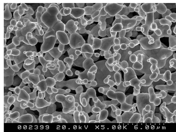
Minimal grain growth and sintering-inhibition achieved with doped W powders.
