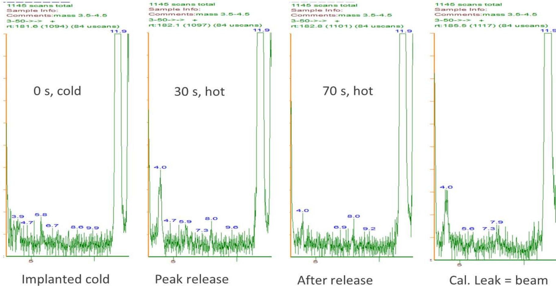
RGA spectra between masses 3 and 12. *Left:* After He beam implantation; *Left-center:* After heating to  $\sim 1000\text{ }^\circ\text{C}$  in 30 s; *Right-center:* 40 s later showing depletion of He from sample. *Right:* Same region with sample cold and calibrated He leak open to chamber.
