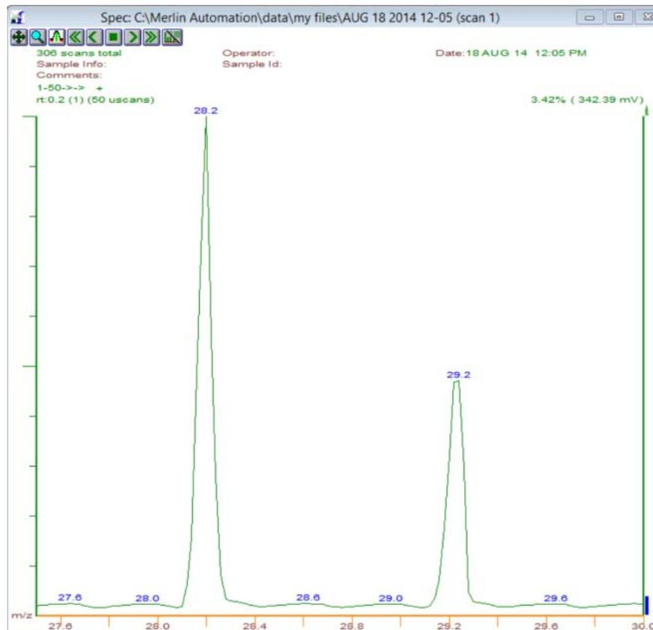
**Left Panel** - Mass 29 ( $^{12}\text{COH} + ^{13}\text{CO}$ ) is larger relative to mass 28 ( $^{12}\text{CO}$ ) in the right panel. The **right panel** was recorded near the peak of the  $^{13}\text{CO}$  release and the left panel 30 minutes later.
