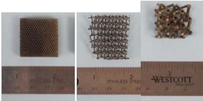
Porous Scaffolds for Refractory Solar Selective Coatings - SuNLaMP
