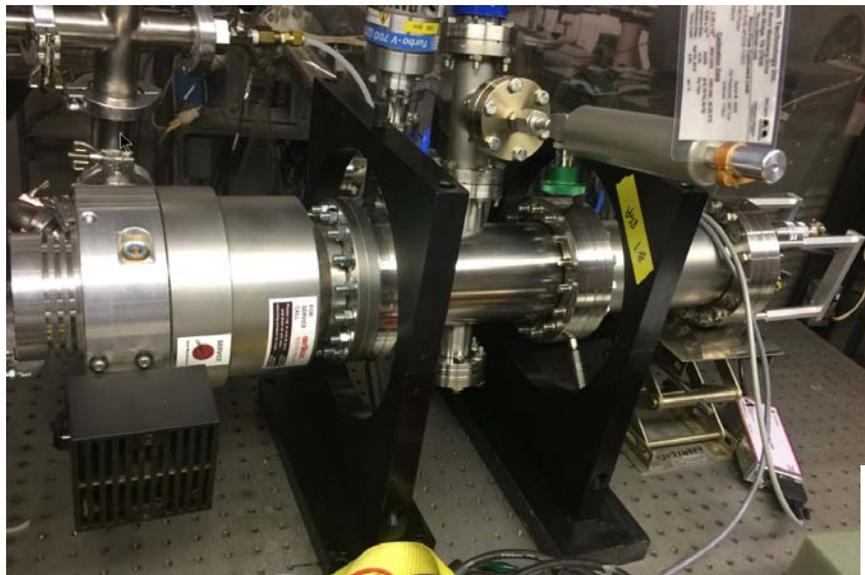
**Upgrade to UHV and much more compact sample chamber and heater. Will add plasma “cleaner” to reduce hydrocarbon background.**
