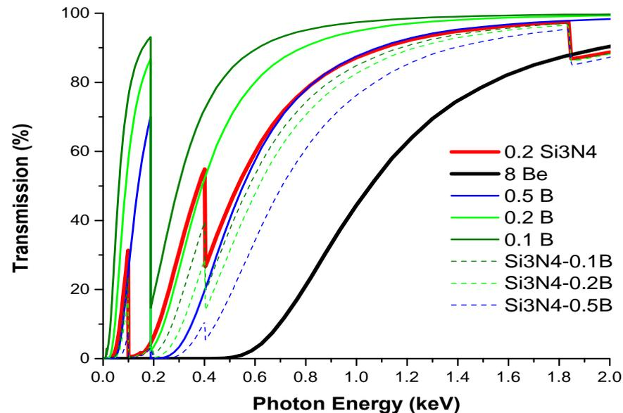
**Figure 1:** A comparison of low energy low energy x-ray transmission of diamond (C) and boron (B) windows of different thicknesses in comparison with standard Be window.
