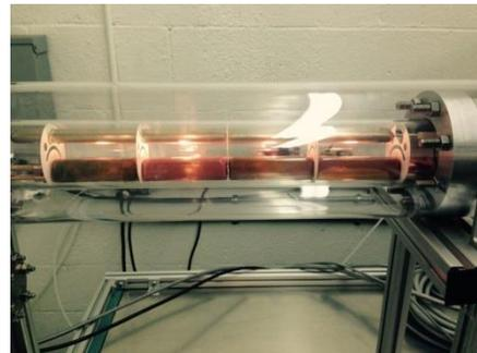
\* 18" long tube built in Phase I with 4 x-ray beams
