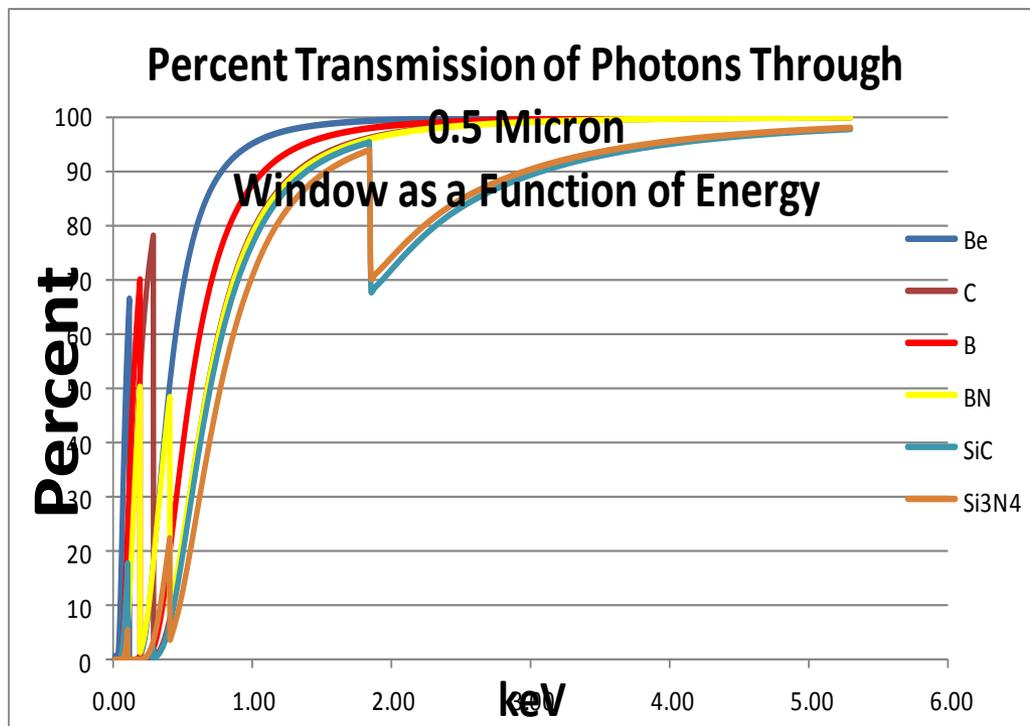
**Figure 2:** Calculated x-ray transmission curves for 0.5micron thick films of various materials at UHV. Please note that even though 0.5 micron thick Be has the best transmission, films/foils thinner than 8 microns cannot be used due to pin-holes and poor strength, which is why we need ceramic films.
