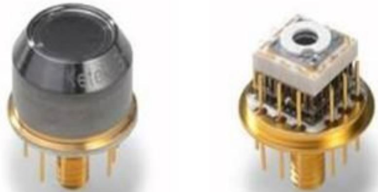
**Figure 5:** Photograph of a sealed x-ray detectors made by Ketek using 9 mm diameter Be window.
