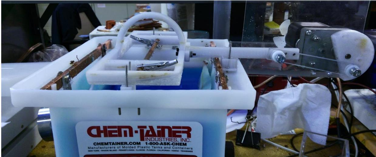
Copper sulfate/sulfuric acid plating bath
