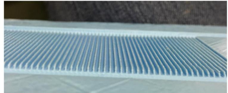
Mold for multi-channel liquid cooled units
