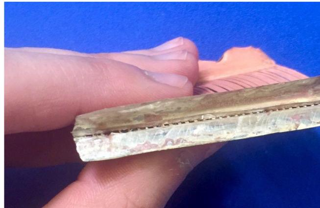
Micro-channel flow regions each measuring 127  $\mu\text{m}$  by 838  $\mu\text{m}$
