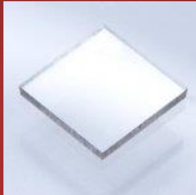
Start with ppm level of nitrogen. Bombard with electrons to make vacancies, then anneal to pair N and V. Add electron to form NV<sup>-</sup>. Single crystal diamonds 5x5x0.5 mm cost about \$600.
