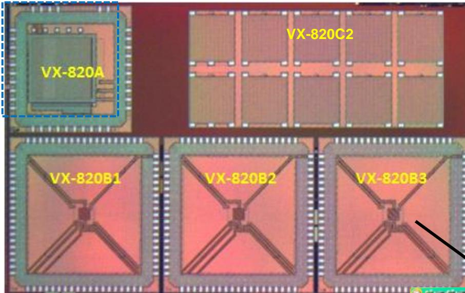
Prototype devices (both SiPM and DSPAD sensors) were evaluated and used in optimization of SPAD element and pixel/readout circuits.
