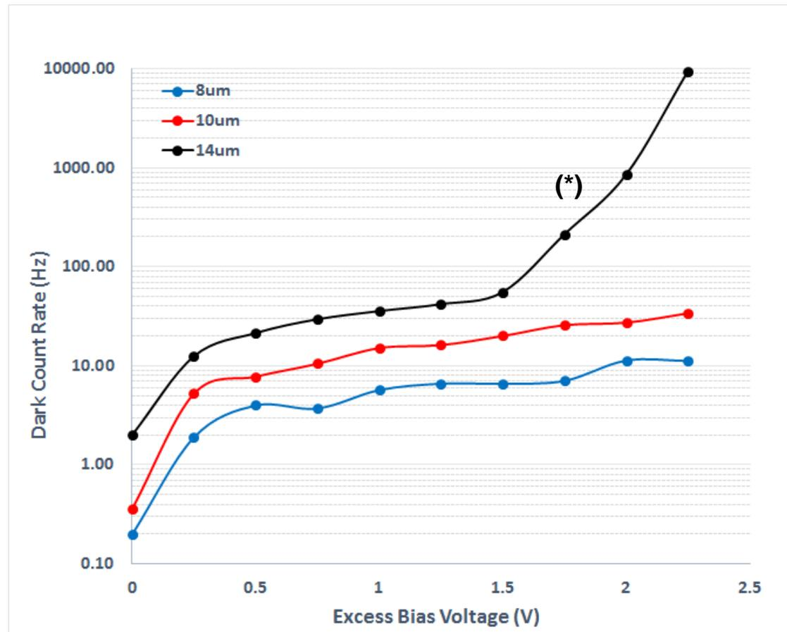
(\*) The 14- $\mu\text{m}$  diameter active area device has a reduced anode to guard ring spacing resulting in an increase in DCR at lower excess bias levels.
