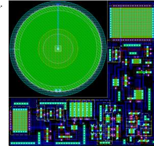
(2) Following active integration or gate time, digital state machine and row control logic scan rows of pixel array sequentially, multiplexing pixel data into column readchain where it is sampled.
