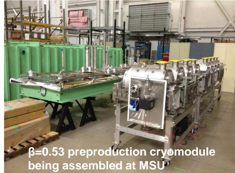
$\beta=0.53$  preproduction cryomodule being assembled at MSU
