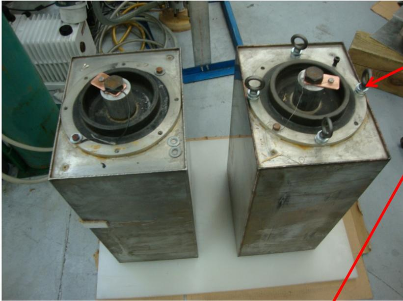
3uF, 100 kV capacitors to be connected in series
