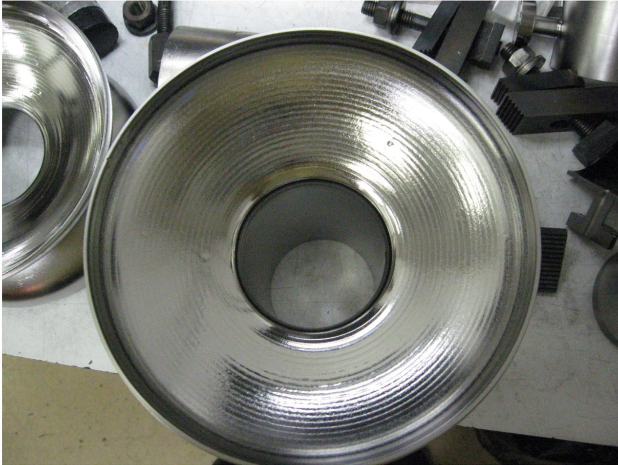
The beam parameters were: 40 mA, 0.5mm diameter beam, travelling at 18 inches per minute, the melting diameter is about 6 mm with a circular pattern at 10 kHz.
