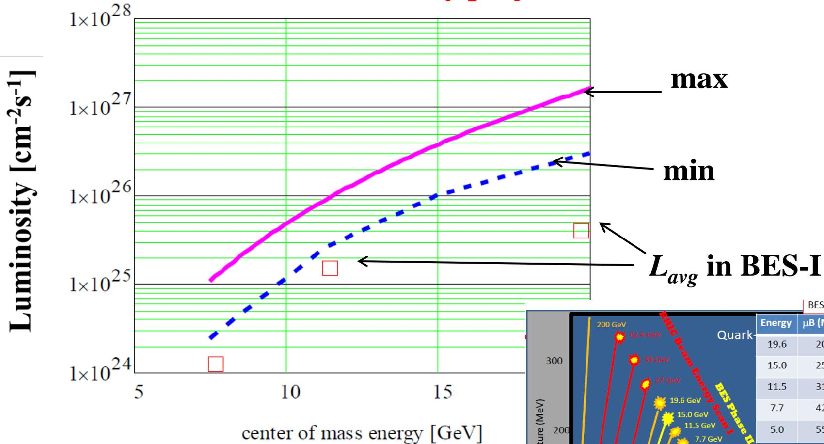
Figure 1. Projection of average store luminosity within +/-1m RHIC with electron cooling. Red squares: measured average line: minimum projection of improvement with cooling. projection of luminosity improvement with cooling.
