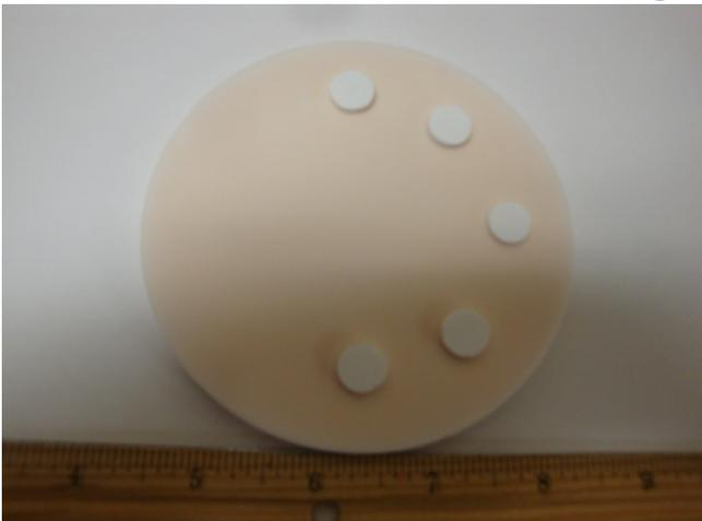
Dye Penetrant Test
